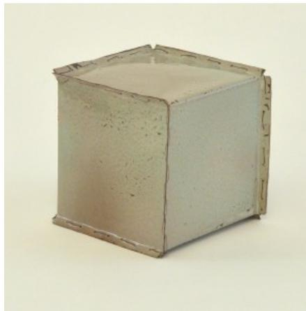
Test piece: sewn 4" copper foil cube, dipped in white liquid enamel 533 from Thompson Enamel Torch: Propane/air Result: fusing achieved quickly with less discoloration than in previous sessions. Some enamel crawling, likely due to over-
