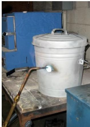
A soldering board was cut to fit within the lid interior. We learned the hard and smoky way that the steel can needed to be sandblasted or sanded prior to firing in order to remove surface coatings that did not approve of fire. Despite the closely mitered bricks, the heat of the torch did not travel well around the interior and enamel vitrification was only achieved on the corner nearest to the torch portal. Sigh.
