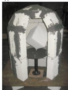
construction and an utter disaster. No amount of indirect firing with an oxy-acetylene torch would coax the enamel into fusing – the interior appeared to be too vast. We even tried bricking up most of the vertical aperture, but to no avail.
