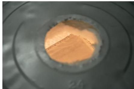
Test piece 1: sewn 10" copper foil cube, white liquid base coat enamel BC 1070 from Thompson, applied by dipping and brushing; Torch: Oxyacetylene with rosebud tip; Result: All-over vitrification, high-fives all around
