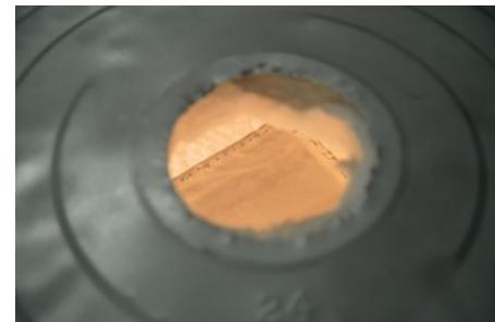
Test piece 1: sewn 10" copper foil cube, white liquid base coat enamel BC 1070 from Thompson, applied by dipping and brushing; Torch: Oxyacetylene with rosebud tip; Result: All-over vitrification, high-fives all around
