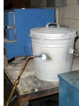
A soldering board was cut to fit within the lid interior. We learned the hard and smoky way that the steel can needed to be sandblasted or sanded prior to firing in order to remove surface coatings that did not approve of fire. Despite the closely mitered bricks, the heat of the torch did not travel well around the interior and enamel vitrification was only achieved on the corner nearest to the torch portal. Sigh.
